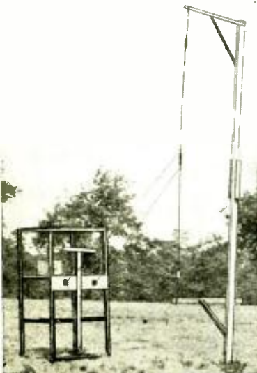
Photo. above, shows the appearance of the "local oscillator" used in making the field intensity measurements. Fig. 5.
