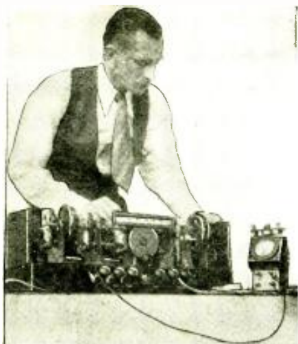
The author making tests on the 14-tube superhet.
