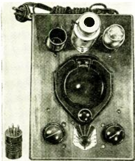
Here's a nifty short-wave converter that works on 110 volts A.C. or D.C. Plug-in coils are used for tuning in the various radio frequency bands. (No. 160)
